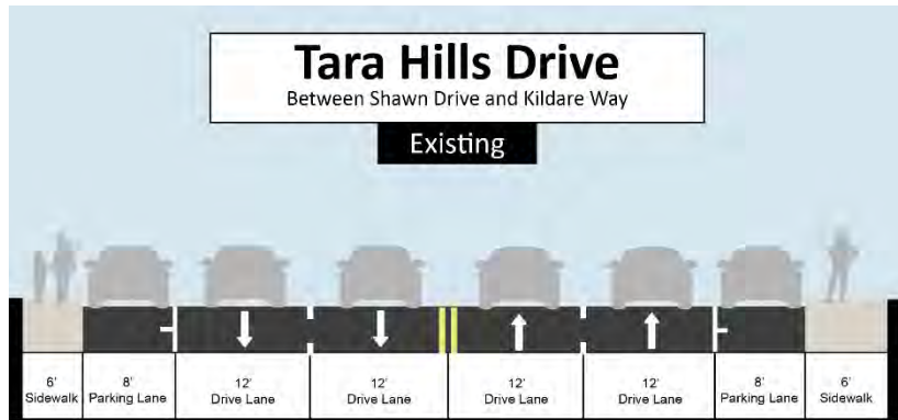
Figure 15: Tara Hills Drive (Arterial Street) Existing Dimensions
