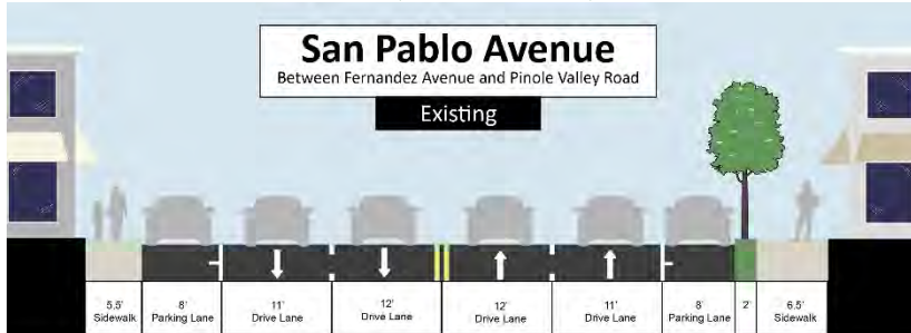
Figure 13: San Pablo Avenue (Arterial Street) Existing Dimensions
