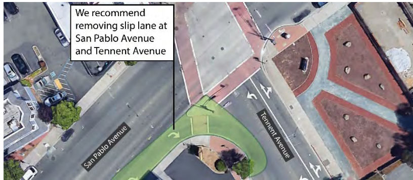
Figure 4: San Pablo Avenue & Tennent Avenue Slip Lane Removal
