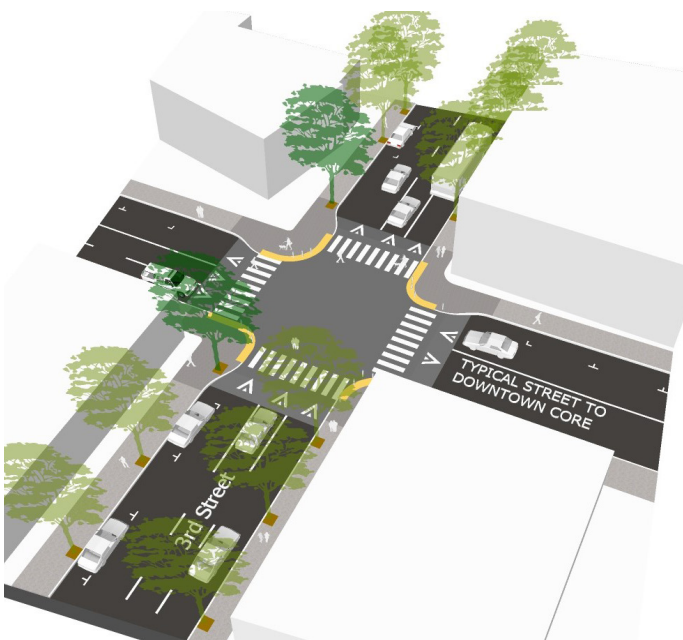
Along Third Street, we are elevating the intersections to reduce the roadway's cross slope to meet ADA criteria.
