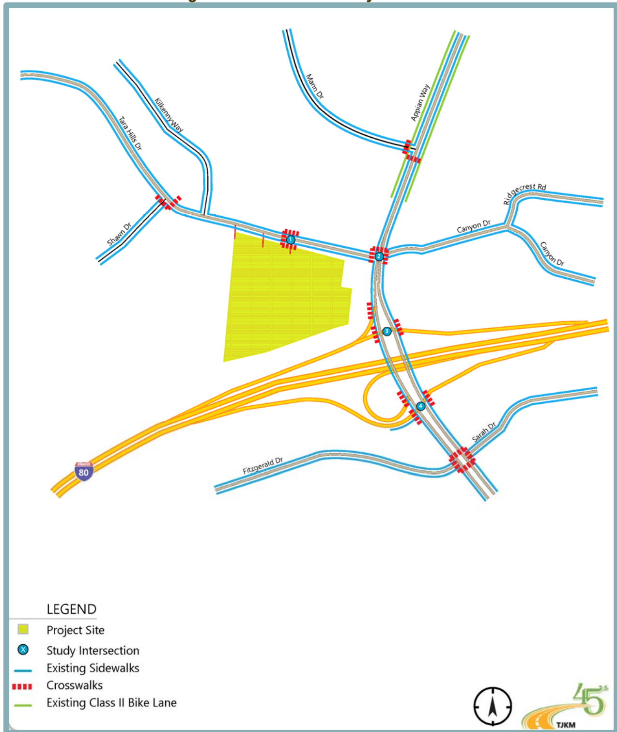
Figure 30 Existing Pedestrian and Bicycle Facilities
