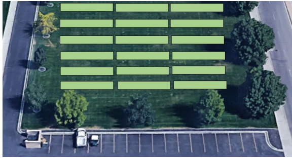
546 panels, 210-kW system
