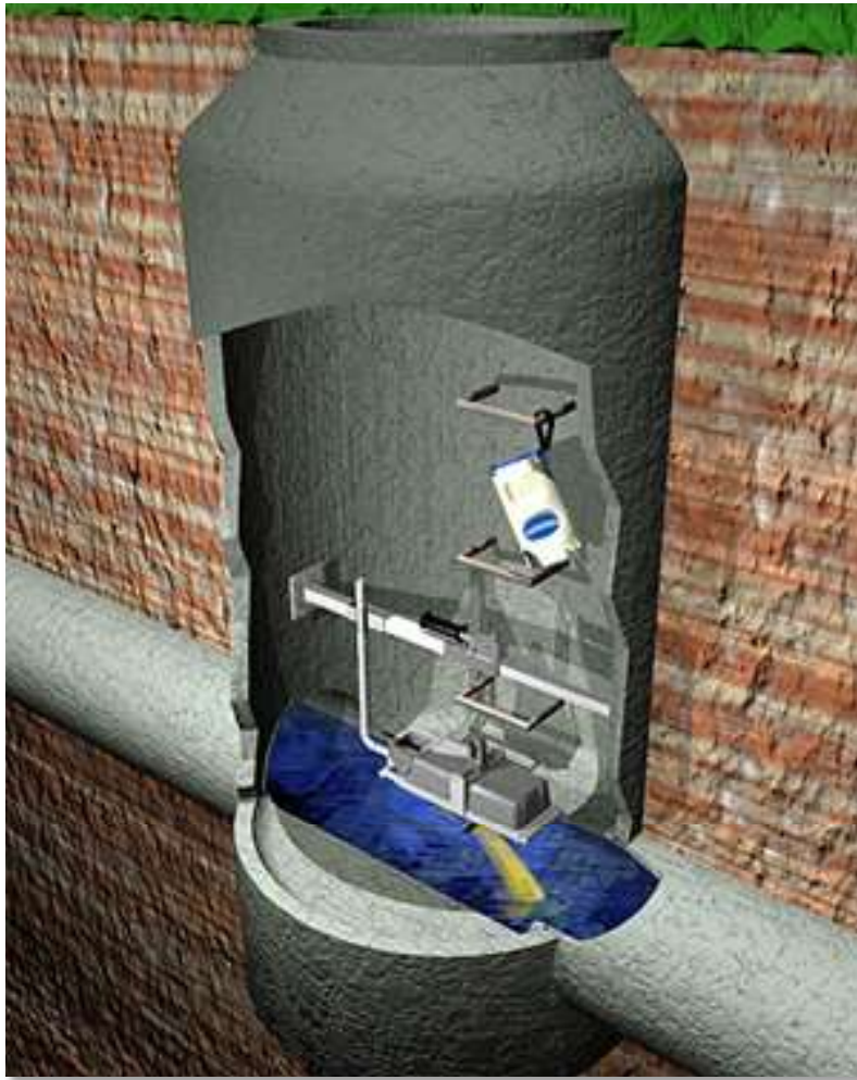
Figure 2-4. Typical Flo-Dar Flow Meter Installation
