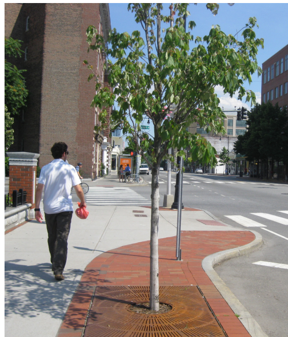
Curb extensions visually and physically narrow the roadway, creating safer and shorter crossings for pedestrians.
